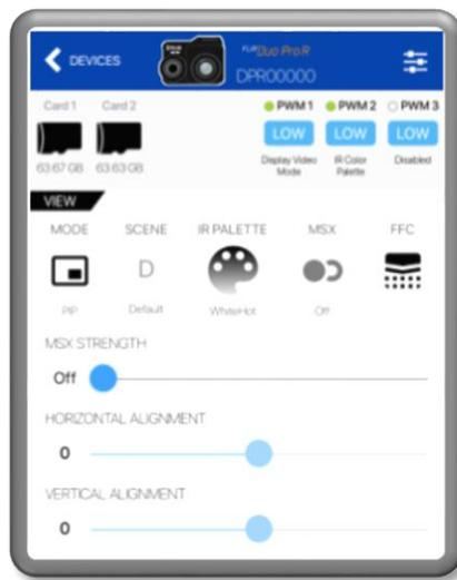
Figure 12. MSX Parameter Adjustment
